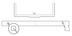
Screw the wall mount brackets on the pen mark; screw the threaded mounting post into the back of the soundbar; then hook the soundbar on the wall.
