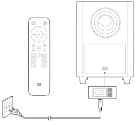
The wireless subwoofer automatically connects with the soundbar when both units are powered on. If the subwoofer is on and connected, the LED lights white continuously.
